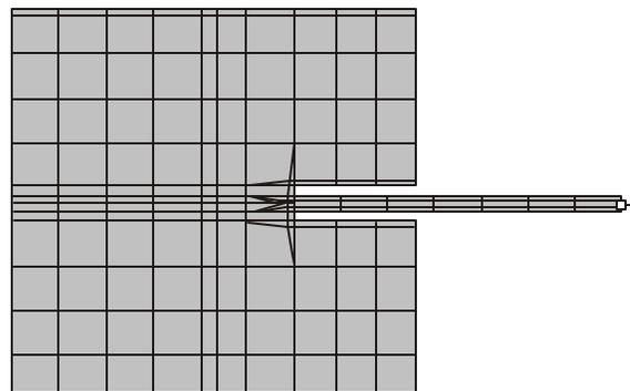
Fig. 2. Meshing result on the antenna.
