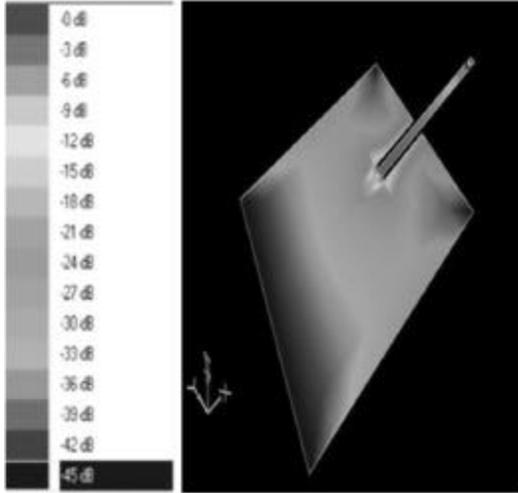
Fig. 6. The current distribution display at 2.18 GHz.
